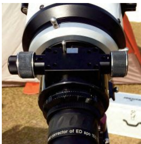
Image 5 - Closeup of the Esprit 150 focuser locking lever.
